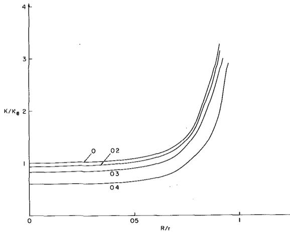
Fig. 7 Error introduced in the inferred value of  $K$  through neglect of both material inertia and plasticity effects in the analysis of experimental data
