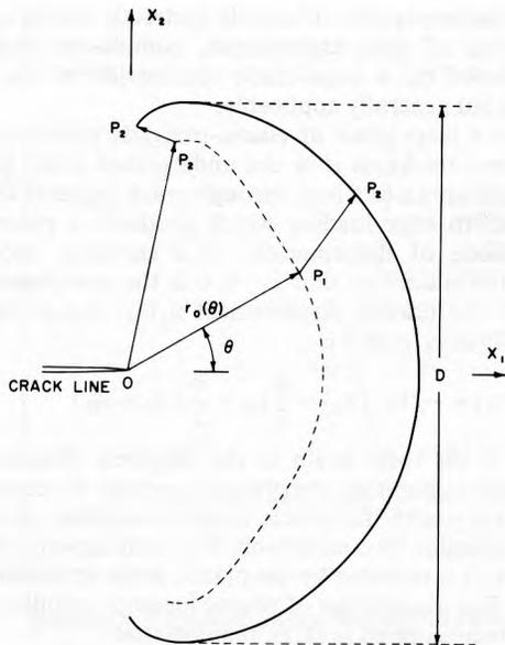
Fig. 3 Geometrical construction of the predicted initial curve (dashed) and caustic curve (solid).
