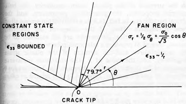
Fig. 2 Angular sectors of the asymptotic elastic-plastic solutions for  $n \rightarrow \infty$  [6]
