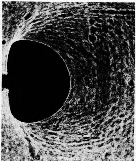
Fig. 4 Photograph of shadow spot, surrounded by slip lines, obtained by reflection from points well within the plastic zone
