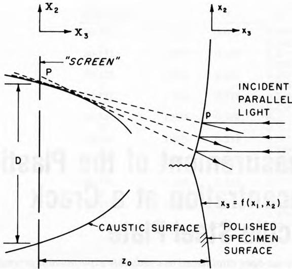
Fig. 1 Schematic of the optical setup for caustics by reflection
