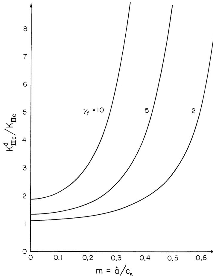
Figure 1. Mode III dynamic fracture toughness as a function of crack tip velocity in an elastic-ideally plastic rate insensitive material, according to the critical plastic strain fracture criterion. (From Freund and Douglas [3].)
