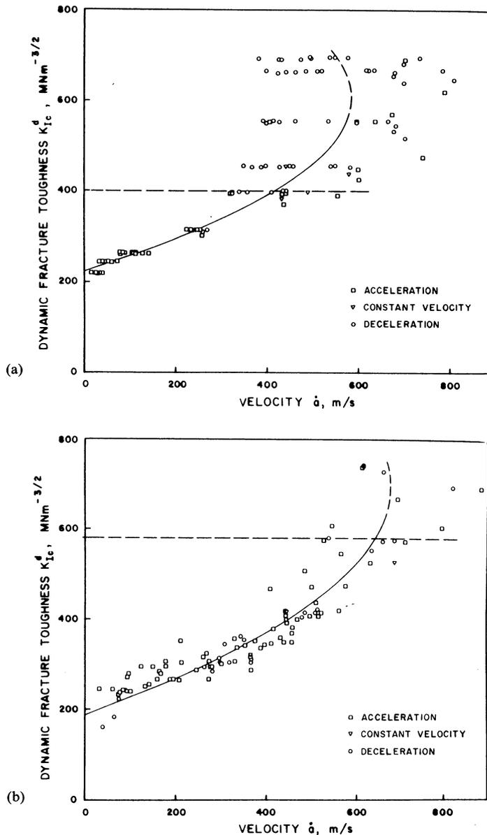
Figure 15. Dynamic fracture toughness as a function of crack velocity for SEN specimens of high strength steel. Specimen dimensions, (a) 60 cm  $\times$  40 cm  $\times$  0.5 mm (b) 160 cm  $\times$  40 cm  $\times$  0.5 mm. Increased scatter in smaller specimen. (From Dahlberg, Nilsson, and Brickstad [54].)
