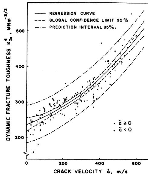
Figure 4. Dynamic fracture toughness as a function of crack velocity for a high strength steel. (From Brickstad [14].)
