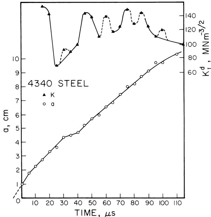
Figure 9. Stress intensity factor and crack length as a function of time for a DCB specimen of 4340 steel. (Rosakis and Zehnder, work in progress, Caltech 1984.)
