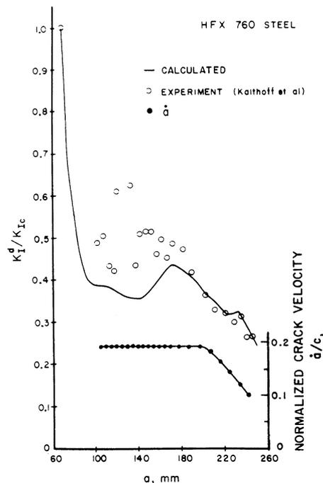
Figure 14. Experimentally determined crack velocity and stress intensity factor (from Kalthoff et al. [53]) and computed stress intensity factor (from Nishioka and Atluri [52]).
