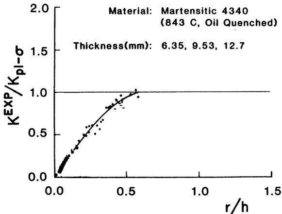
Figure 12. Static stress intensity factor as determined by caustics, divided by plane stress value for different distances,  $r$ , from the crack tip. (From Rosakis and Ravi-Chandar [44].)
