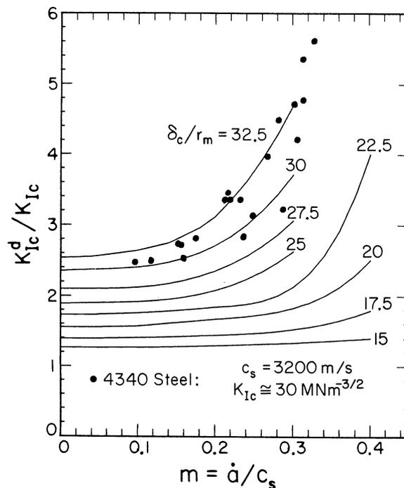
Figure 2. Mode-I dynamic fracture toughness as a function of velocity according to the critical crack tip opening angle fracture criterion. Also included are experimental results of Rosakis, Freund and Duffy [13] for 4340 steel. (From Lam and Freund [2].)
