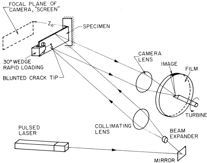
Figure 11. Experimental set-up for reflected, high speed photography of caustics. (Rosakis and Zehnder, work in progress, Caltech 1984.)
