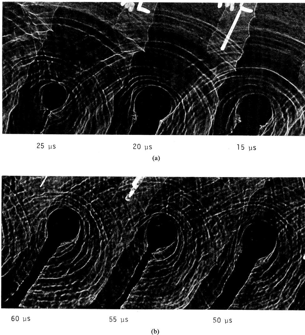
Figure 10. Reflected caustic patterns corresponding to dynamic crack growth test recorded in Fig. 9 for 4340 steel. (a) Strong dynamic effects are demonstrated by visible unloading waves and oscillations in caustic diameter. (b) Visible oscillations in the width of wake indicate vibrations of the cantilever arms of DCB specimens. (Rosakis and Zehnder, work in progress, Caltech 1984.)
