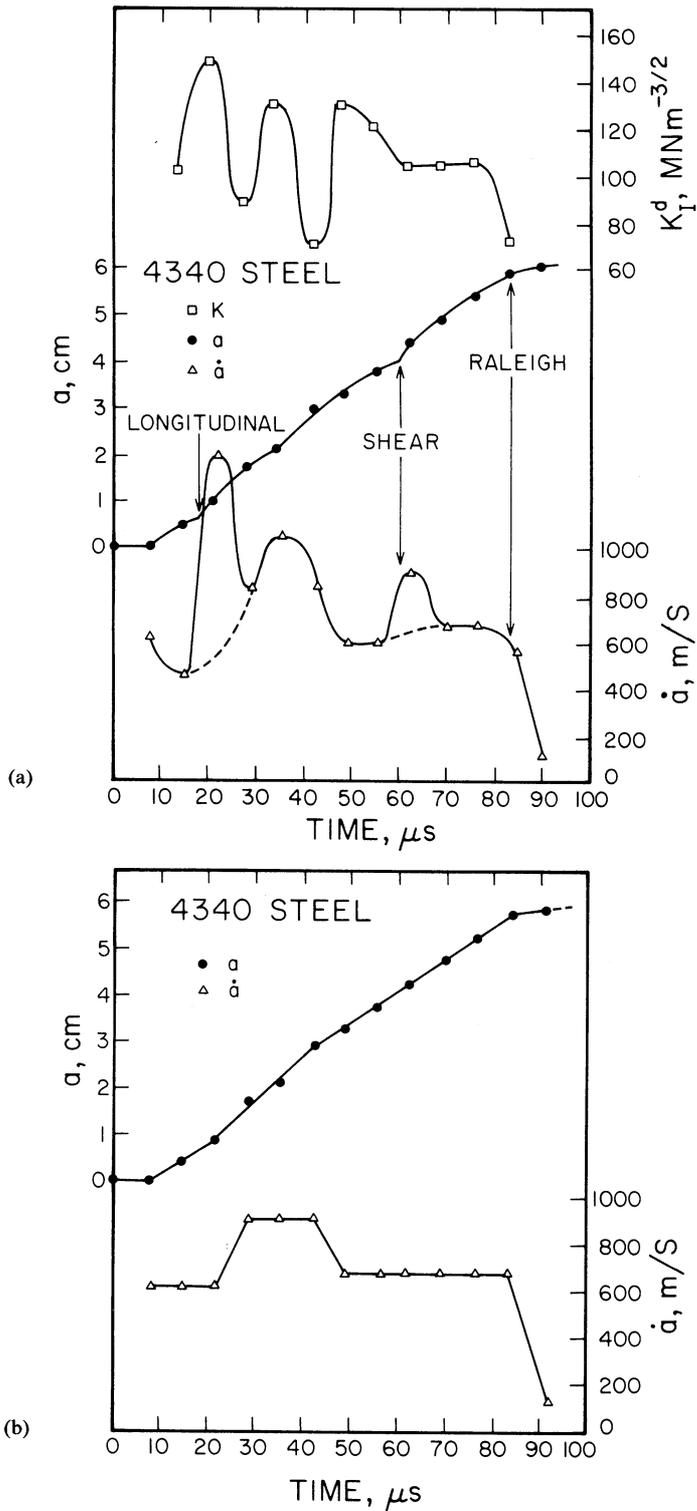
Figure 13. (a) Stress intensity factor, crack length and crack velocity as functions of time. Arrows indicate reflected stress wave arrivals. (b) Alternative interpretation of  $a(t)$  record. (Rosakis and Zehnder, work in progress, Caltech 1984.)
