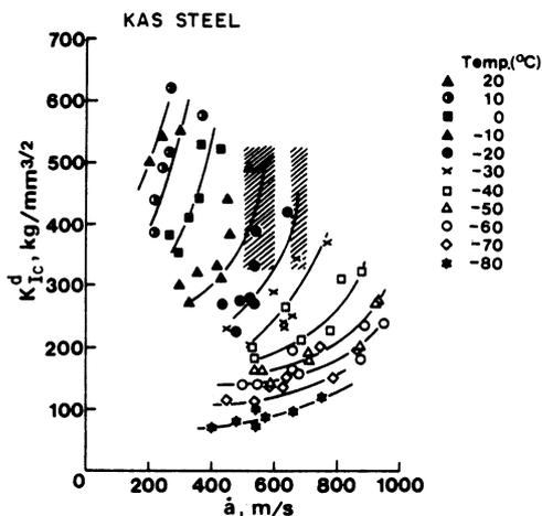
Figure 6. Dynamic fracture toughness as a function of crack velocity for different temperatures.  $100 \text{ kg mm}^{-3/2} = 31 \text{ MNm}^{-3/2}$ . (From Kanazawa et al. [22].)
