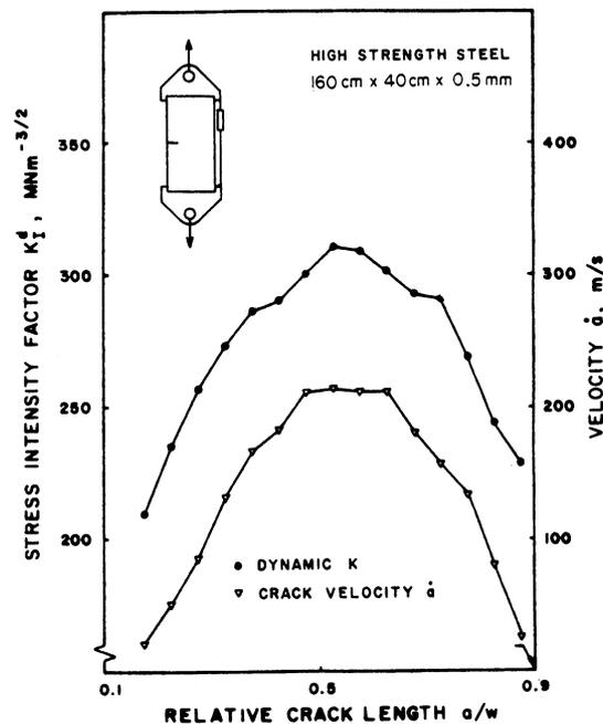
Figure 3. Stress intensity factor and crack velocity as functions of crack length. (From Brickstad [14].)
