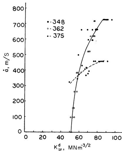
Figure 8. Dynamic fracture toughness as a function of crack velocity for a 4340 steel. (From Kobayashi and Dally [37].)
