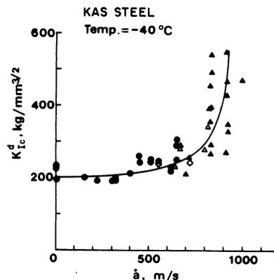
Figure 7. Dynamic fracture toughness as a function of crack velocity at  $-40^\circ\text{C}$ . (From Kanazawa et al. [22].)
