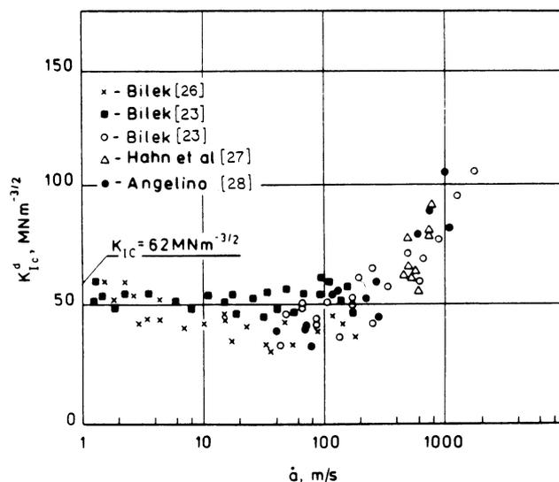
Figure 5. Dynamic fracture toughness as a function of crack velocity for 4340 steel. (From Bilek [23].)
