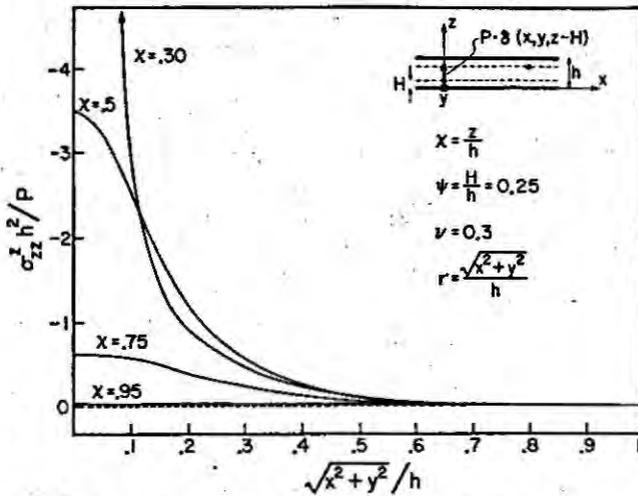
Fig. 2. Variation of the normalized stress  $\sigma_{zz}^* h^2/P$  vs the normalized in-plane distance  $r' = \sqrt{(x^2 + y^2)}/h$ .
