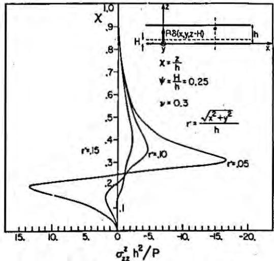
Fig. 4. Variation of the normalized stress  $\sigma_{zz}^* h^2/P$  vs the normalized distance  $\chi = z/h$  measured from the lower surface of the layer. Different curves correspond to  $r' = 0.15$ ,  $r' = 0.10$ ,  $r' = 0.05$ .
