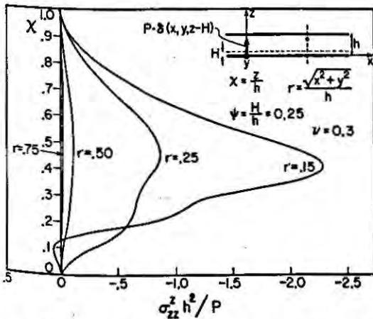
Fig. 3. Variation of the normalized stress  $\sigma_{zz}^* h^2/P$  vs the normalized distance  $\chi = z/h$  measured from the lower surface of the layer. Different curves correspond to  $r' = 0.75$ ,  $r' = 0.50$ ,  $r' = 0.25$ ,  $r' = 0.15$ .
