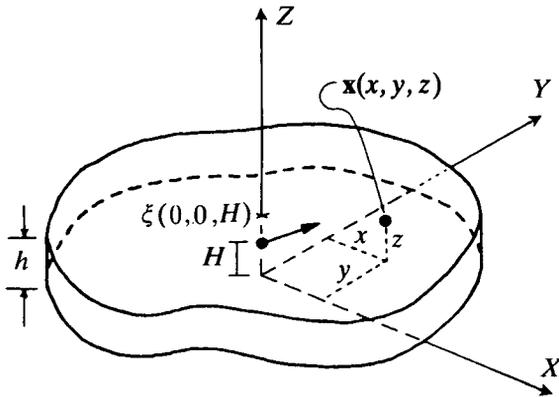
FIG. 1. Single layer with unit internal load applied to a given point. The point  $\mathbf{x}$  is an arbitrary internal point
