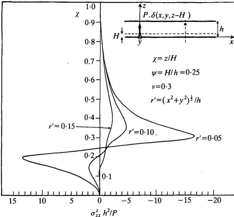
FIG. 4. Variation of the normalized stress  $\sigma_{zz}^2 h^2/P$  versus the normalized distance  $\chi = z/h$  measured from the lower surface of the layer. Different curves correspond to  $r' = 0.15$ ,  $r' = 0.10$ ,  $r' = 0.05$
