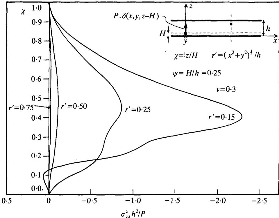
FIG. 3. Variation of the normalized stress  $\sigma_{zz}^z h^2/P$  versus the normalized distance  $\chi = z/h$  measured from the lower surface of the layer. Different curves correspond to  $r' = 0.75$ ,  $r' = 0.50$ ,  $r' = 0.25$ ,  $r' = 0.15$
