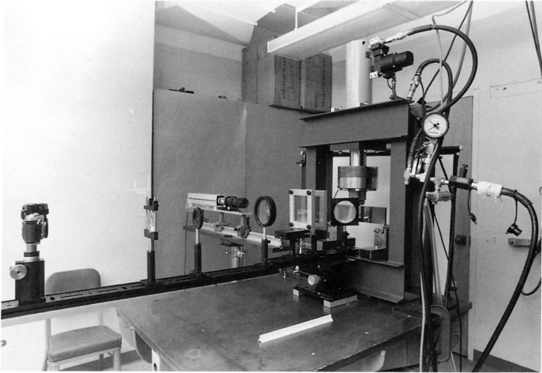
Fig. 6. Experimental arrangement for fracture experiment using CGS.
