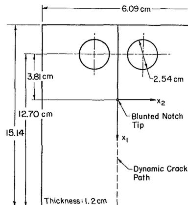
Fig. 1 Specimen geometry
