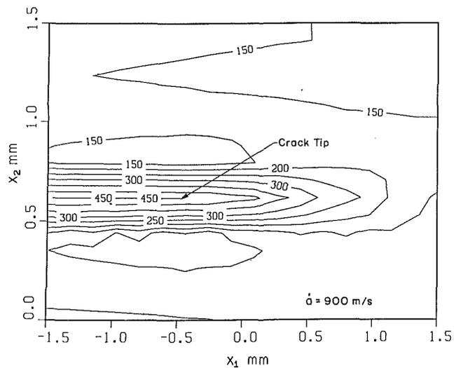
Fig. 4 Contours of equal temperature rise at the vicinity of the propagating crack. Temperature increase is in °C.
