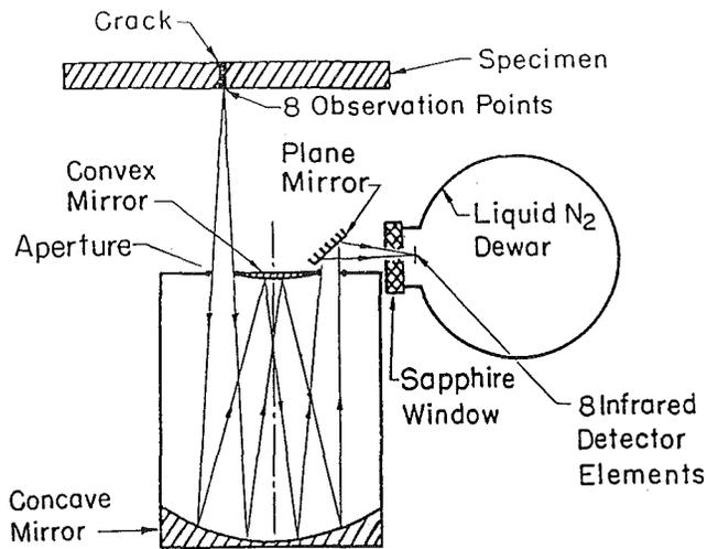
Fig. 2 Schematic of the experimental set-up. The top shows the focusing of radiation onto the infrared detectors. The bottom shows the location of measurement areas relative to crack line.
