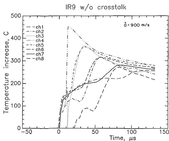
Fig. 3 Temperature rise versus time for each detector element
