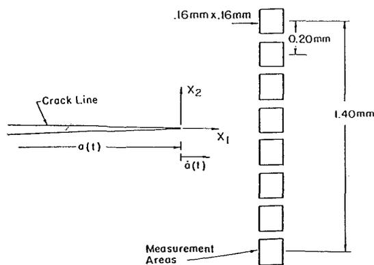
Fig. 2 Schematic of the experimental set-up. The top shows the focusing of radiation onto the infrared detectors. The bottom shows the location of measurement areas relative to crack line.
