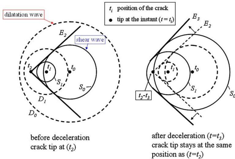
Fig. 25. Wave mechanisms before and after a crack decelerates from intersonic to subsonic speeds where  $t_i$  denotes the time,  $D_i$  and  $S_i$  are the dilatational wave and shear wave radiated from the crack tip at  $t_i$ , respectively, and  $E_i$  is the envelop of all shear wave fronts at  $t_i$ .
