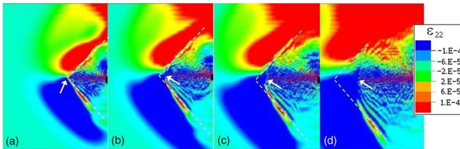
Fig. 24. Intersonic crack propagation deceleration—contours of the strain perpendicular to the crack path where the white arrow indicates the crack tip position in each figure. (a)  $t = 1.4e-5$  (s), (b)  $t = 1.6e-5$  (s), (c)  $t = 1.7e-5$  (s) and (d)  $t = 1.95e-5$  (s).
