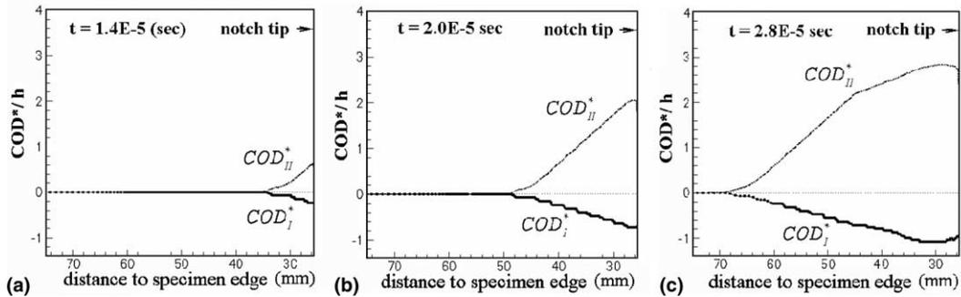
Fig. 14. A numerical example of mode I and II opening profiles during propagation, where  $h$  is the thickness of the bonding layer; in (c) the I, II, III, IV refer to the contact zones illustrated in Fig. 11.
