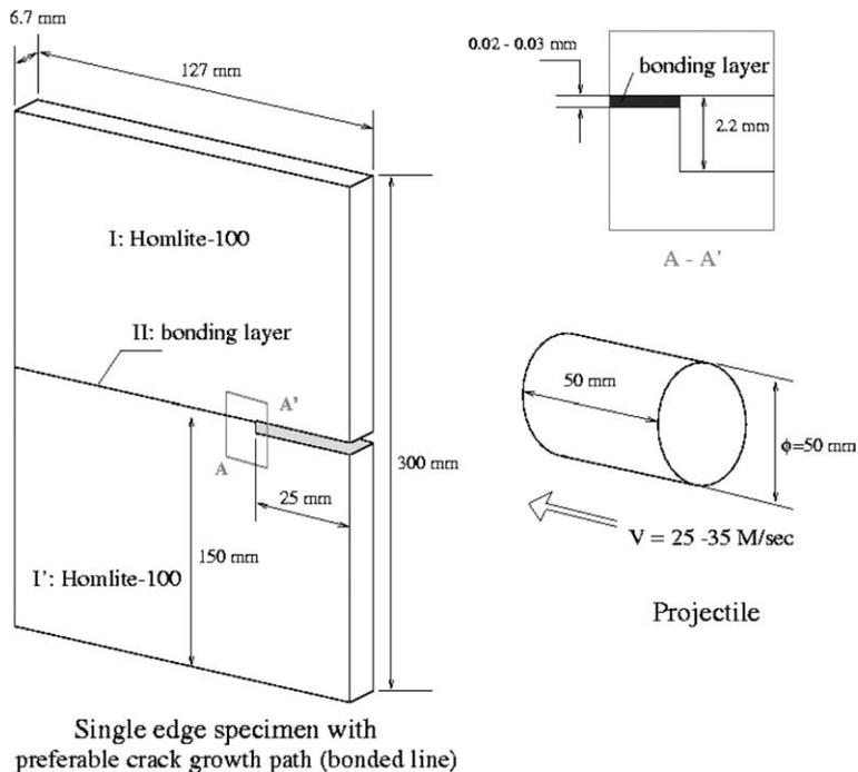
Fig. 1. Caltech mode II dynamic fracture test.
