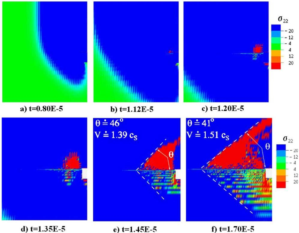
Fig. 7. Fracture process zone initiation and subsequent crack propagation. (a)  $t=0.80e-5$ , (b)  $t=1.12e-5$ , (c)  $t=1.20e-5$ , (d)  $t=1.35e-5$ , (e)  $t=1.45e-5$  and (f)  $t=1.70e-5$ .
