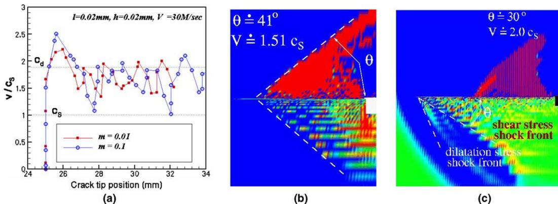
Fig. 20. Intersonic and supersonic crack propagations. (a) Speed vs. crack growth for two simulations with different strain rate hardening power. (b) The stress shock for case with  $m = 0.01$ . (c) The stress shock for case with  $m = 0.1$ .
