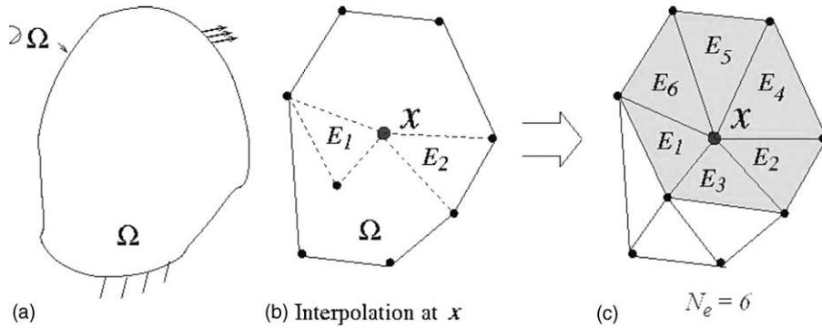
Fig. 6. (a) A boundary value problem defined on  $\bar{\Omega}(= \Omega \cup \partial\Omega)$ . (b) An approximated solution at  $\mathbf{x}$  can be obtained from either element  $E_1$  or  $E_2$ . (c) MPFEM approximation—an average from the surrounding elements.
