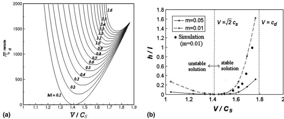
Fig. 23. (a) Relationship between propagation speed  $V$  and  $\bar{v}_d^{\text{remote}}$ , theoretical solution (Hao et al., in press); (b) comparison between predictions and present numerical solutions.
