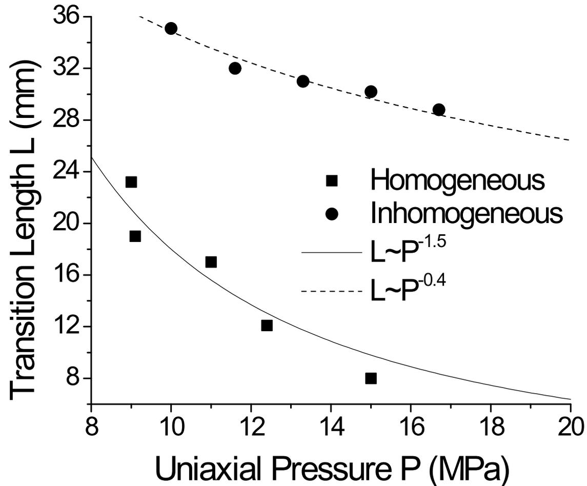
*For the same load, it takes longer propagation distance in bimaternal to transition to super shear*
