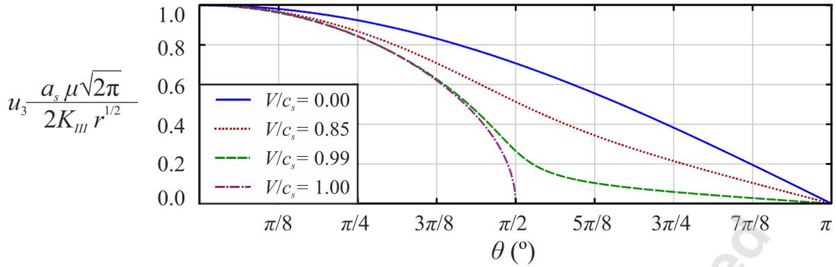
Figure A.1. The Normalized mode III classic elastodynamic displacement (considering the parameter  $a_s$ ) A region with zero displacement appears as the velocity reaches the limiting velocity  $V/c_s$ .
