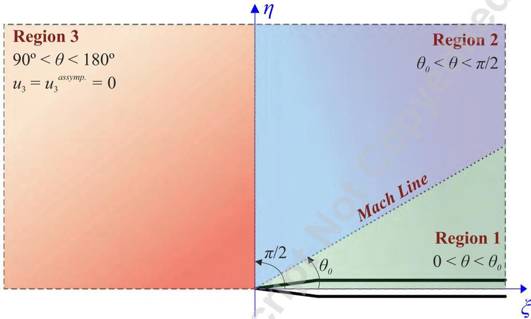
Figure 7. The 3 different regions that appear asymptotically close to the crack-tip ( $\sin \theta_0 = 1/\sqrt{\lambda}$ ) that are also suggested by FEM solution.
