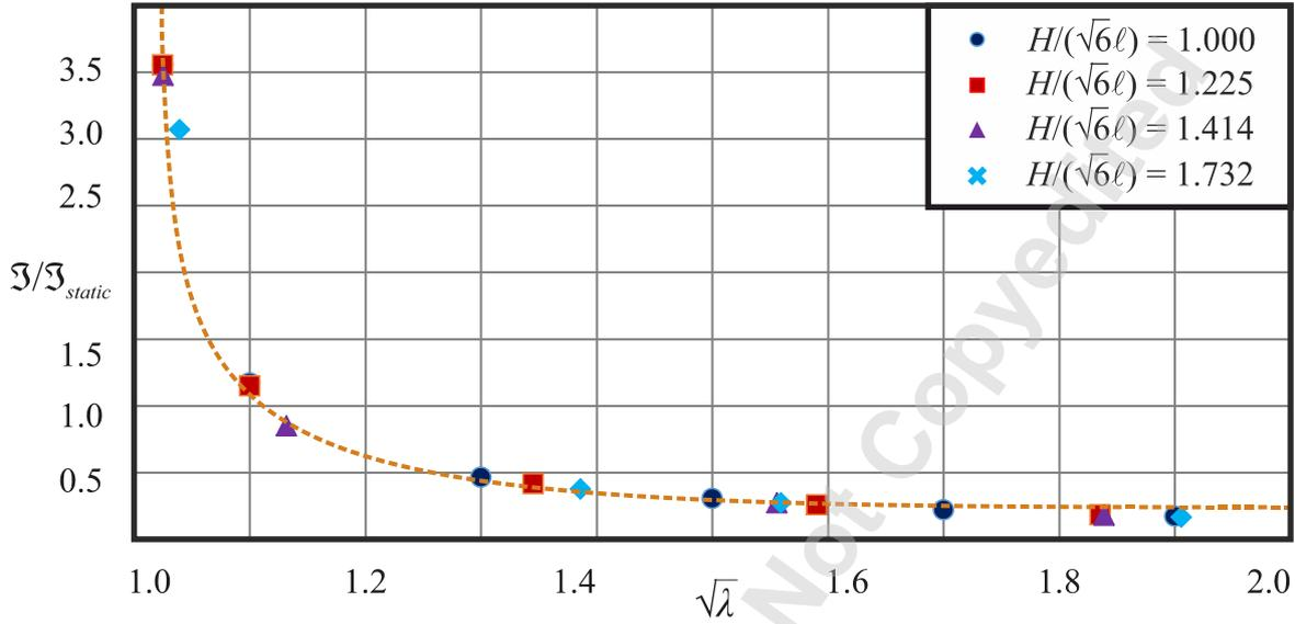
Figure 16. The normalized J-integral with respect to the static case, where the results show the combined influence of  $V/c_s$  and  $H/(\sqrt{6}\ell)$  in the parameter  $\sqrt{\lambda} = (HV)/(\sqrt{6}\ell c_s)$  for  $\tau_0/\mu = 4.00 \cdot 10^{-2}$ , and  $L/(\ell/\sqrt{2}) = 6.667$ .
