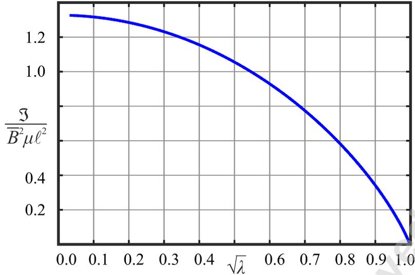
Figure 12. The normalized energy release rate for the elliptic (sub-Rayleigh) case ( $0 \leq \lambda < 1$ ).
