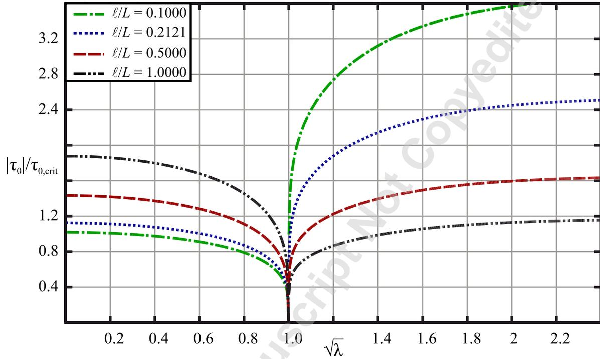
Figure 17. The approximate normalized shear stress with respect to the critical shear, for which crack starts to propagate. For a specific shear stress, crack tip accelerates and it is possible to jump to super-shear rupture.
