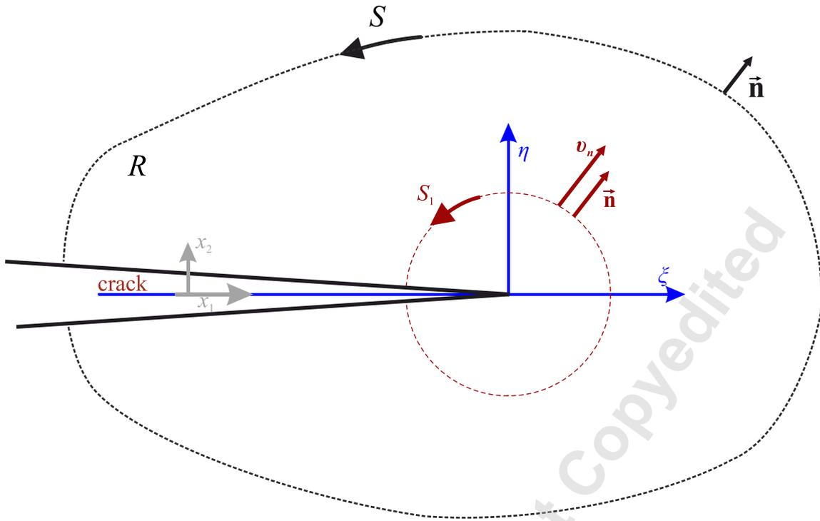
Figure B.1. The crack tip configurations at a certain time instant.  $(x_1, x_2)$  is the fixed coordinate system and  $(\xi, \eta)$  is the coordinate system moving with the crack-tip.
