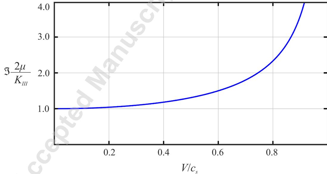
Figure A.2. The mode III J-Integral for the classic elastodynamics (sub-shear) case
