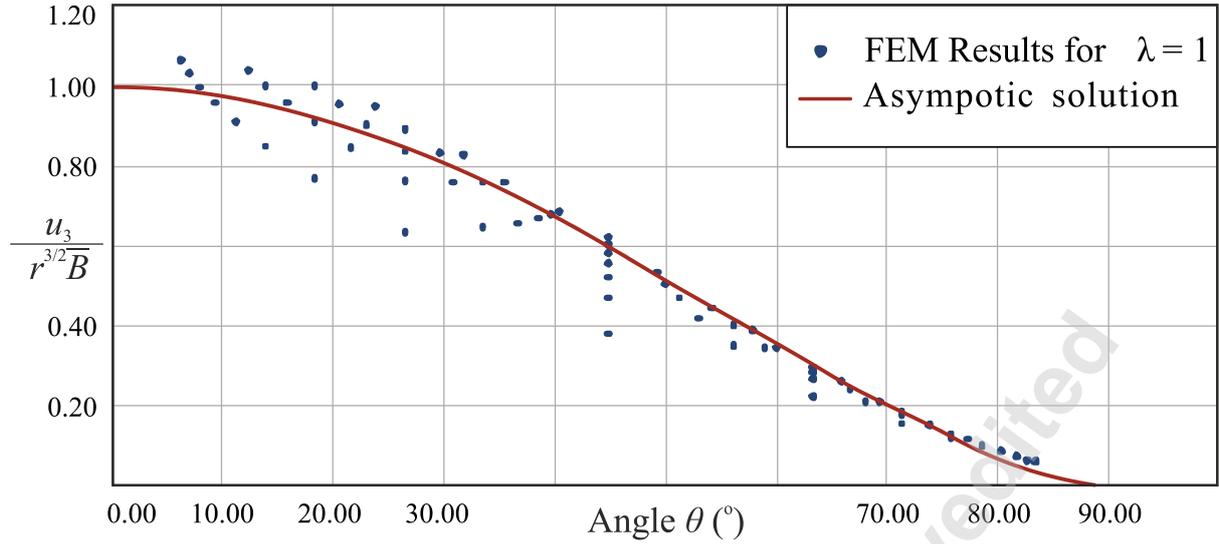
Figure 9. The asymptotic solution for  $\lambda = 1.00$  according to the FEM and its theoretical estimate (28) for  $\tau_0 / \mu = 4.00 \cdot 10^{-2}$ .
