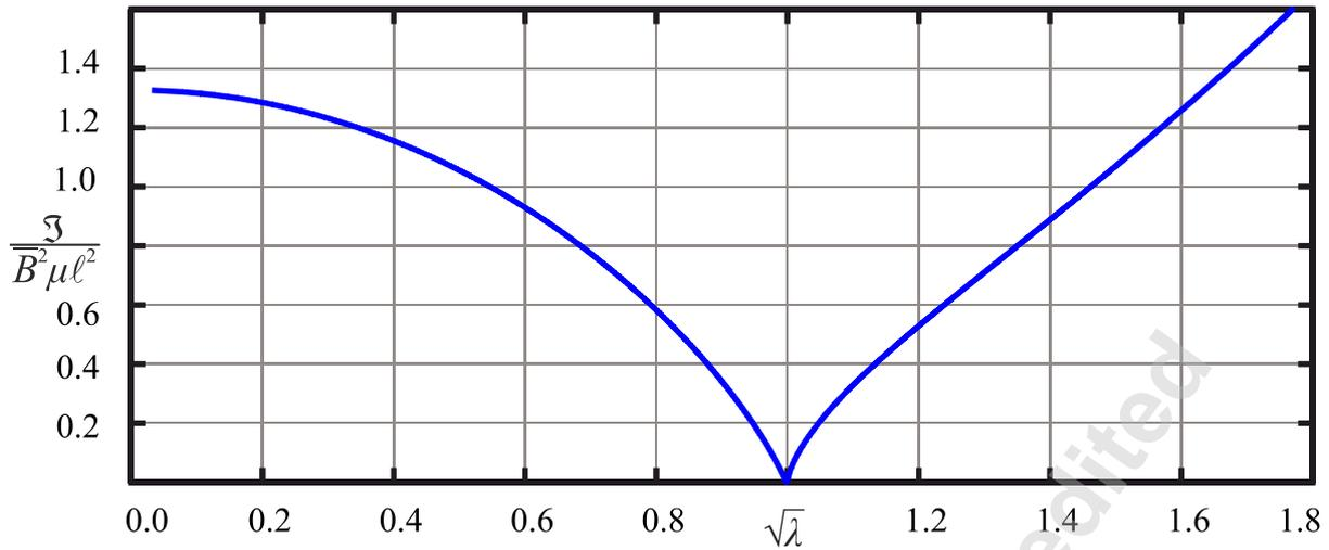
Figure 14. The normalized energy release rate for the anti-plane mode III fracture in a flexoelectric material.
