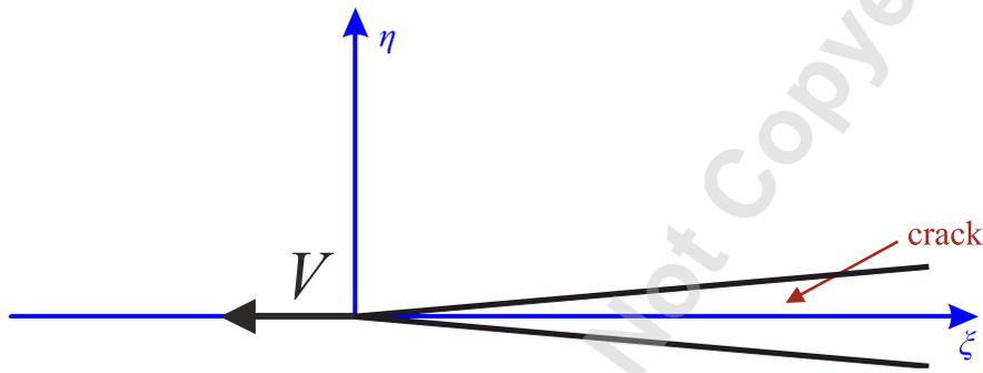
Figure 1. The motion of the steady state mode III fracture with rupture velocity  $V$ .
