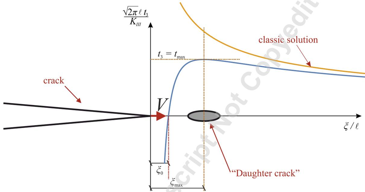
Figure 18. Schematic of a Burridge – Andrews type of dynamic crack advance based on [13]. Note that the classic solution holds outside our present solution.
