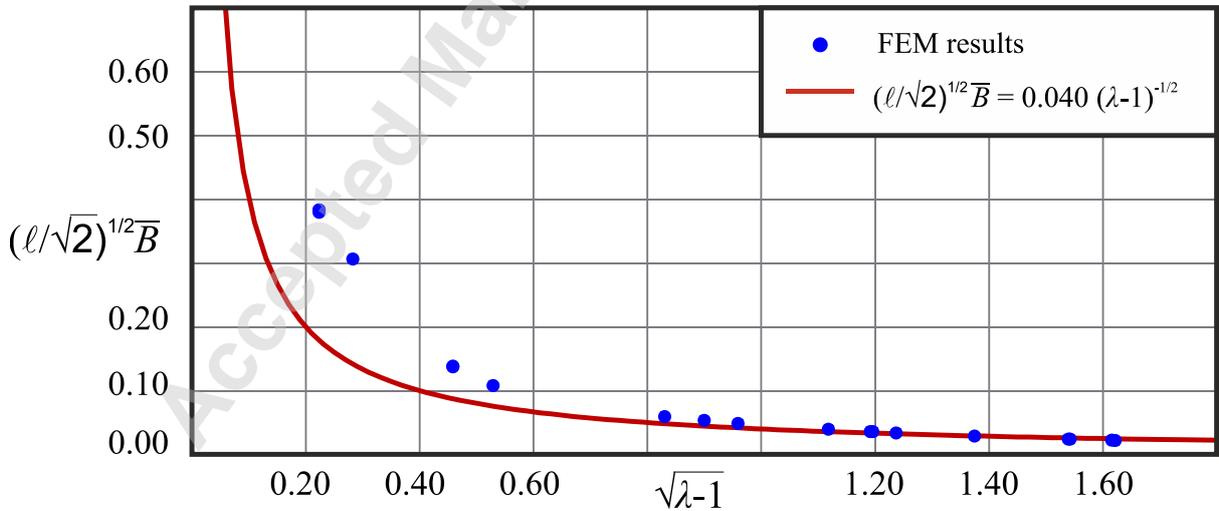
Figure 10. The numeric values of the parameter  $\bar{B}$  in the hyperbolic problem according to the results close to the crack-tip finite element analysis, for  $\tau_0 / \mu = 4.00 \cdot 10^{-2}$ .
