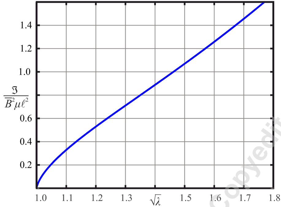
Figure 13. The normalized energy release rate for the hyperbolic mode III steady state crack  $\lambda = (H^2 V^2) / (6l^2 c_s^2)$ .
